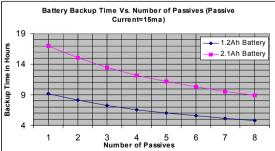
**NOTE:** Calculations made for **Avanti Compact** with onboard keypad using a **neon** sounder, assuming 1 complete alarm cycle of 20 minutes.
